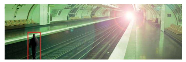
IQ-100 uses a highly sophisticated form of video motion analytics to protect an area from intrusion whilst detecting abnormal behavior such as loitering,running and objects travelling in the incorrect direction. The software continuously tracks the movement of objects across the screen. A virtual tripwire or region is drawn on the screen and whenever this perimeter is breeched the event is recorded and an alarm raised.
